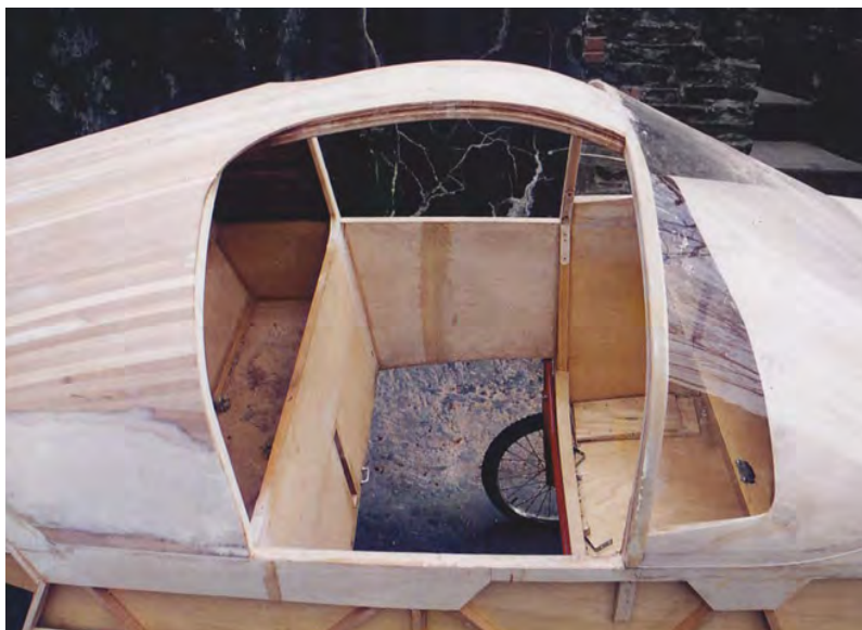
Door cutout saved for forming acrylic glazing
